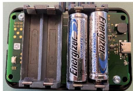
4. Electronics and housing cover (with the information given on the nameplate) form a unit. The same cover must be placed on the electronics again. Then fix the screws again (maximum torque 1.0Nm).
