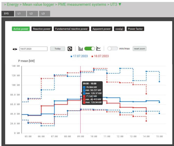
As an alternative a line display can be selected, in which also the display of minimum and maximum values can be activated. This way the fluctuation of the measurements can be seen best.
