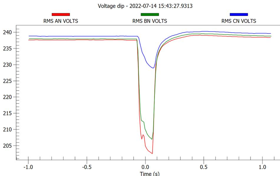
Representation of a voltage dip using PQDiffactor
