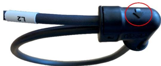
The individual current modules in the ring are connected using SMA connection cables.
