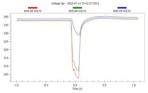
Representation of a voltage dip using PQDiffractor
