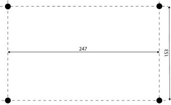
Drilling plan for field housing
