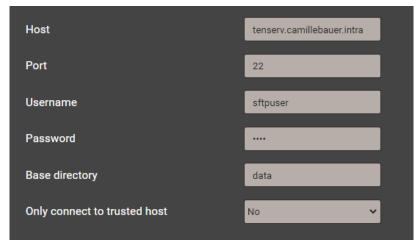
For improving security, you may select that the device connects to trusted hosts only. When activating this setting the host must be present and sends a public key back to the device. If you accept this key the associated host will be added to the list of trusted servers.
