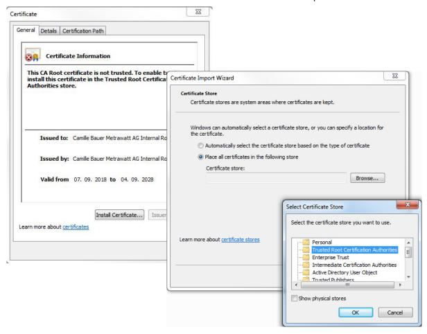
The imported certificate is valid for all devices of the PQ, AM, DM and CU series. Agree to install the certificate if the below security warning appears:
