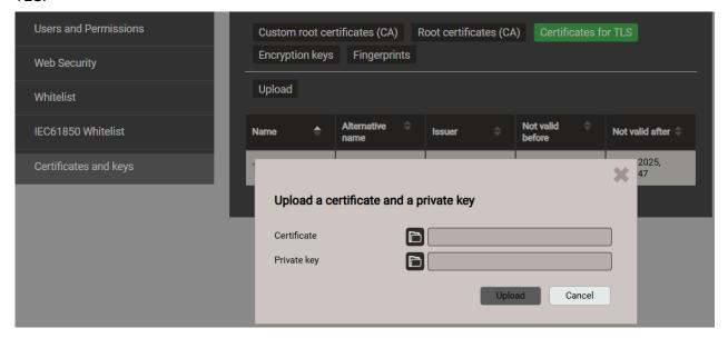
The uploaded certificate can then be selected when activating the HTTPS communication via *Settings* of the *Security System* in the menu *Web Security*.
