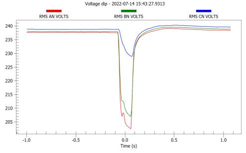
Representation of a voltage dip using PQDiffractor
