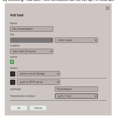
The task "24h\_PowerMeans" will generate daily CSV files containing standard mean-values for the past 24 hours.
