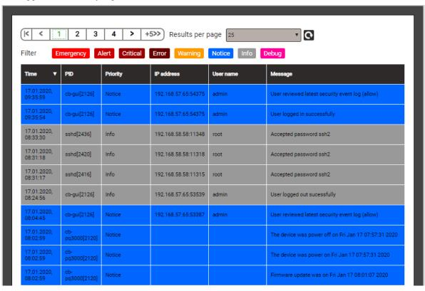
Example of a security log: The severity of each message is shown in a color code, which may also serve as filter criteria.
