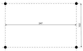
Drilling plan for field housing
