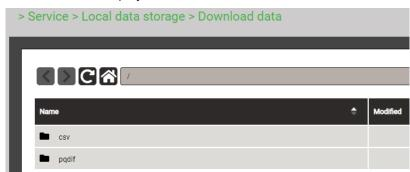
Files in the **pqdif** folder are stored in a hierarchical time structure (year, month, day). By selecting the desired date and double-clicking on the appropriate file, a PQDIF may be easily downloaded.
