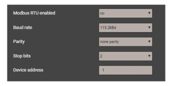
A proper operation requires that all devices connected to the bus have equal communication settings (baud rate, transmission format) and unique device addresses. Use the appropriate menu in the settings of communication.
