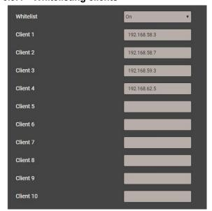
It is possible to define a list of IPv4 and/or IPv6 addresses of up to 10 clients allowed to have access to the device. All other clients will be blocked. Enable the whitelist via the Settings of the Security system in the item Whitelist.
