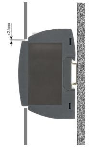
The **PQ5000CL-1** / **-2** with display can also be mounted that the front of the device protrudes through a cut-out in the enclosure. So, the operating buttons and the display become accessible. With centric mounting using the below maximum cut-out a gap between enclosure and device results, which does not exceed 2.5mm on each side.
