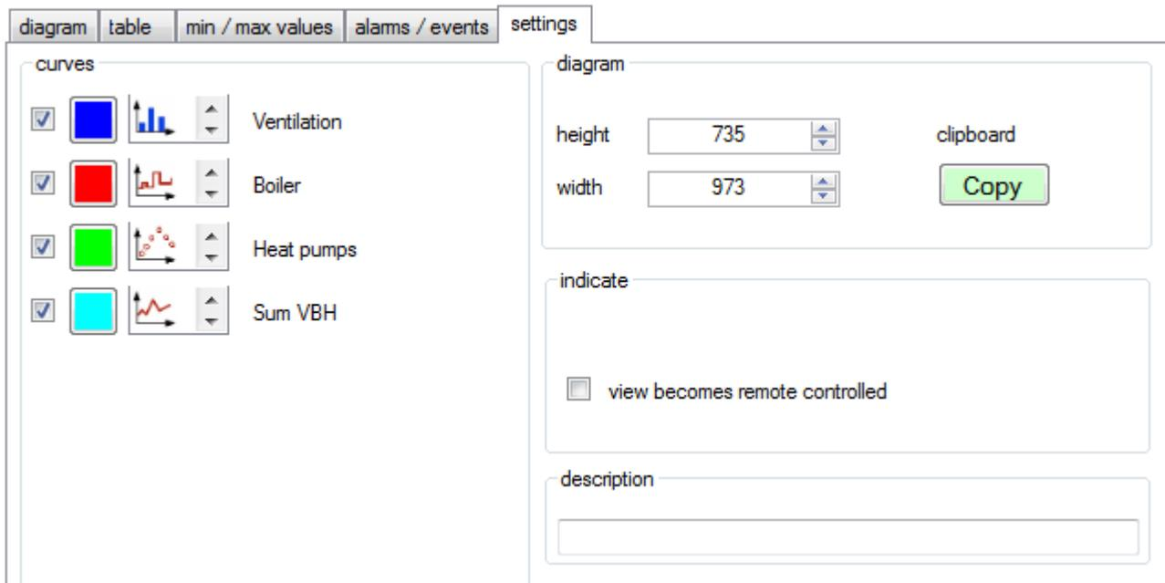
**curves:** For each individual measurement the display may be switched on or off. The colour of each curve can be modified by selecting the coloured rectangle. As well the form of the display can be selected by choosing your preferred type from the list.
