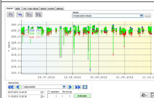
In the graphical measurement display you first have to change the display mode to “measured values”.
