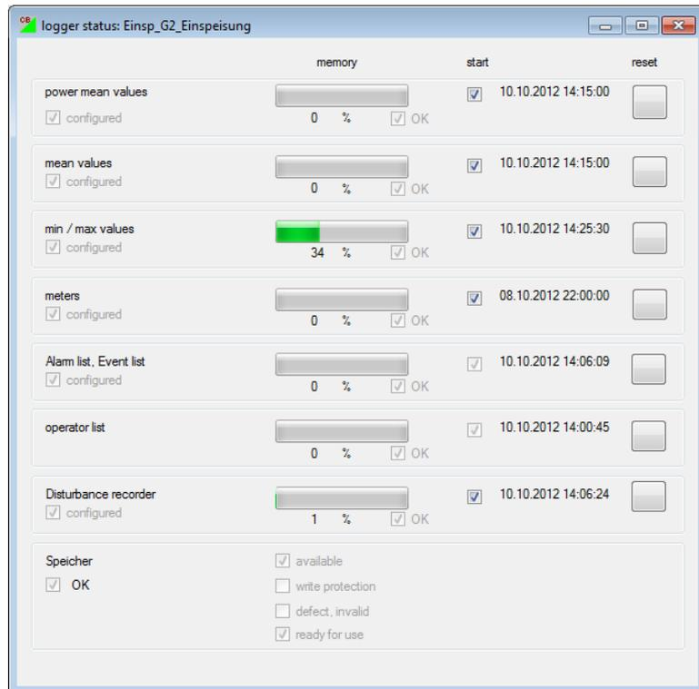
Only for the *APLUS* also the memory state is available. Because for the *APLUS* a mobile data memory (SD card) is used, you can and have to monitor its state additionally. If for example the SD card is removed during normal operation, the complete recording process of the data logger is stopped, because there is no internal memory for temporary storage available.
