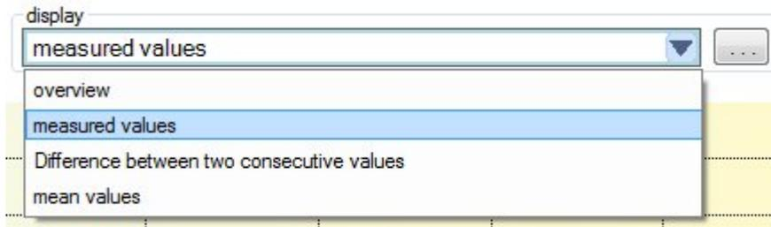
**overview:** (default) The time needed is decreased by displaying minimum, maximum and mean-value of multiple points only. This setting should be activated during the search for parts of interest. It should not be activated during final analysis.
