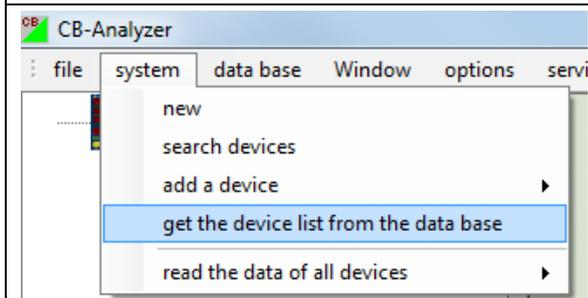
To analyze reports the device list must be created from the data base, because for virtual devices no data access is possible.
