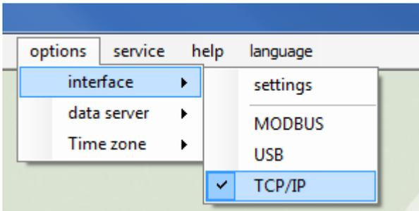
The communication interface is designed the same way as for the CB-Manager. The search for devices therefore delivers the same result. Therefore also devices without data logger will be found or devices with data logger from which data can't be read because the required protocol is not supported by the selected interface.
