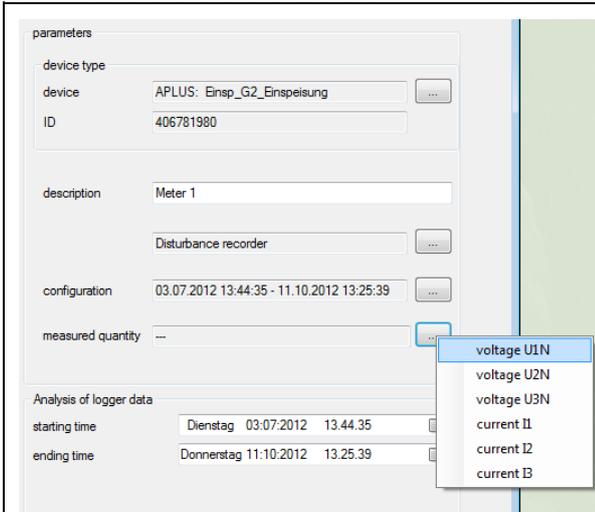
In the opposite example the disturbance recordings consists of data sets of all phase to neutral voltages and all phase currents.
