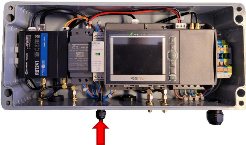
For device variants with separate power supply, the housing must be opened for connection by removing the 4 screws on the top of the housing. The diameter of the supply cable through the cable gland to the input terminals can be 3.5 up to 7 mm.
