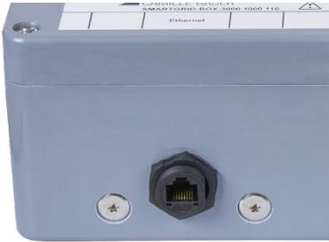
**Hint:** Ex-works the LAN socket of the RUT241 inside the device is connected to the Ethernet socket of the Smart Grid Box and the WAN socket of the RUT241 is connected to the base unit. Please verify if point 2) is not working.
