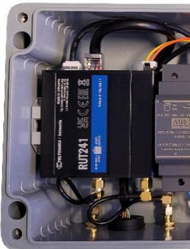
The router is mounted on the left side panel. To insert the SIM card, follow the 6 steps shown below.
