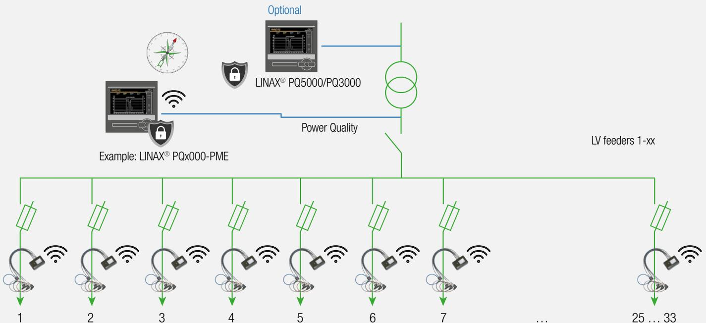
Base station with SINEAX® AM, SINEAX® DM, LINAX® PQ or CENTRAX® CU series, incl. integrated Power Monitoring Energy Module (PME) and PME sensors for acquisition of max. 100 currents via radio signal.
