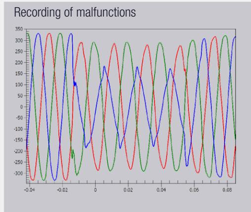
All voltages are monitored for disturbances, such as dip, interruption or swell. These incidents are registered as events. A statistical evaluation is not required because there is no limitation for such events.
