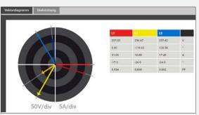
Phasor diagram to control connections
