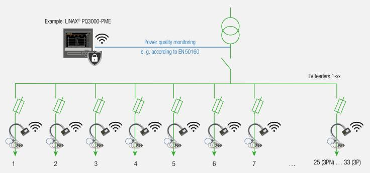
Base station with SINEAX<sup>®</sup> AM, SINEAX<sup>®</sup> DM5000, LINAX<sup>®</sup> PQ or CENTRAX<sup>®</sup> CU series, incl. integrated Power Monitoring Energy Module (PME) and PME sensors for acquisition of max. 100 currents via radio signal.
