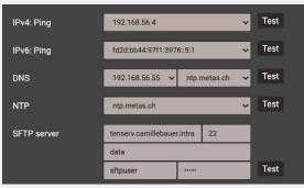
Communication tests: Control of network structure
