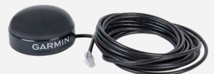
GPS receiver for time synchronisation
