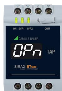
The display is intended to show the current TAP number. It is configurable. e.g. if max taps are set at 25 and if input range of resistance is 0 - 25k Ohms, then a 1k change in input will be reflected by 1 TAP change on the display. i.e. for this case, for 0 input, TAP number will be 0, for 1k input, TAP number will be 1, for 2k input, TAP number will be 2, and likewise.
