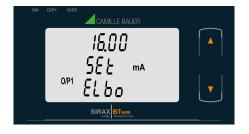
Confirmation of Elbow value Pressing the " Down" key will re-enter into the " Elbow value edit" mode.
