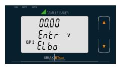
Pressing the " Down" key will enter the "Output 2 Elbow value edit " mode.
