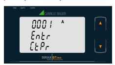
Pressing the " Down" key will enter the transducer into "CT Primary value edit" mode.
