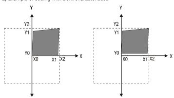
X0 = Start value of input Y0 = Start value of output X1 = Elbow value of inputY1 = Elbow value of output
