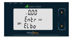
Pressing the " Down" key will enter the " Output 1 Elbow value edit" Mode.
