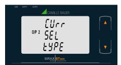
Pressing the " Down" key will enter the "output 2 type edit" mode and scroll between voltage and current.
