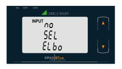
Pressing the " Down" key will enter the " Elbow enable or disable edit" mode and scroll the value between yes and no.
