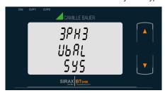
Pressing the " Down" key will enter into the "System Type edit" mode. For Active / Apparent / Reactive Power Transducer, System type will scroll between
