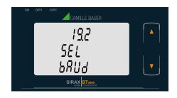
This screen allows the user to set Baud Rate of RS 485 port. The values displayed on screen are in kbaud.
