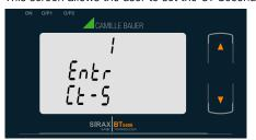
Pressing the " Down" key will enter transducer into "CT Secondary value edit" mode.
