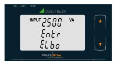
Pressing the " Down" key will enter into the "Input Elbow value edit" mode.
