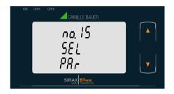
Pressing the " Down" key will enter into the "Parity & stop bit edit" mode and scroll the value between
