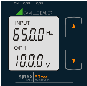
Screen 3: Voltage Input and Output 1 as Voltage
