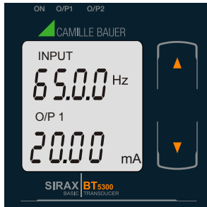
Screen 4: Voltage Input and Output 1 as Current
