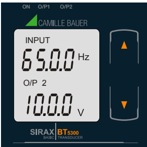
Screen 5: Voltage Input and Output 2 as Voltage
