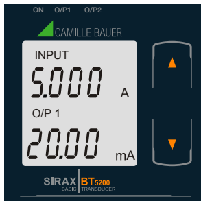
Screen 4: Current Input and Output 1 as Current
