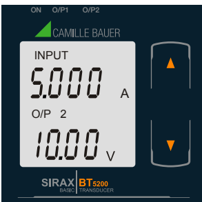
Screen 5: Current Input and Output 2 as Voltage
