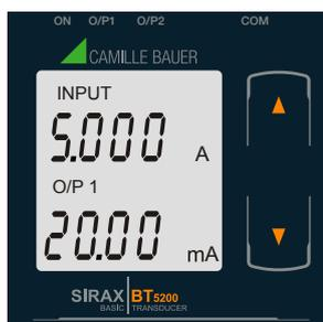
Screen 4: Current Input and Output 1 as Current
