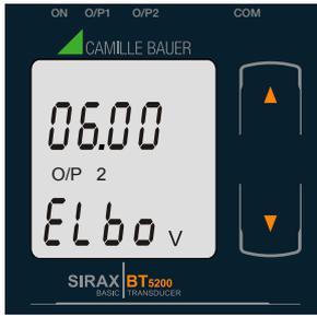
Pressing the “
