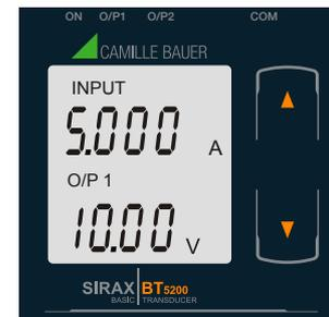
Screen 3: Current Input and Output 1 as Voltage
