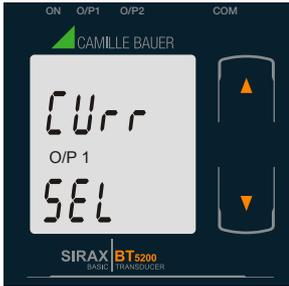
Pressing the “
