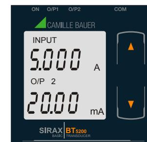
Screen 6: Current Input and Output 2 as Current
