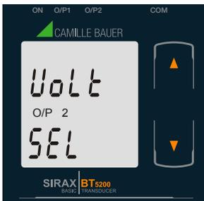
Pressing the “
