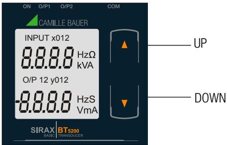
SIRAX BT5200 can be configured and programmed at site for the following: CT Primary, CT Secondary (5A or 1A), Input parameters (i.e start, end and elbow value of Input) and Output parameters (i.e as Voltage or as Current and start, end and elbow value of outputs).
