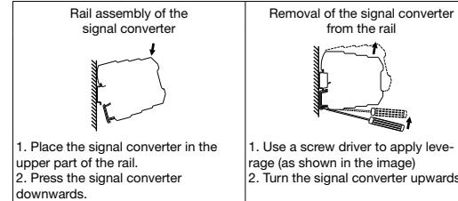
To achieve improved ventilation, we recommend installing the signal converter in a vertical position. Avoid the installation of the signal converter above heat-generating devices. We recommend the installation in the lower part of the control cabinet.
