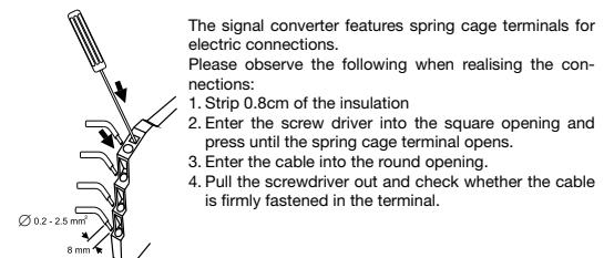
The signal converter features spring cage terminals for electric connections.
