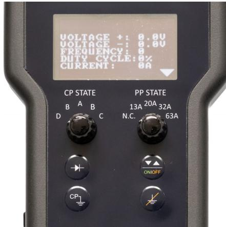
Figure 4: Membrane Keypad with Control Panel, Rotary Switches and Screen
