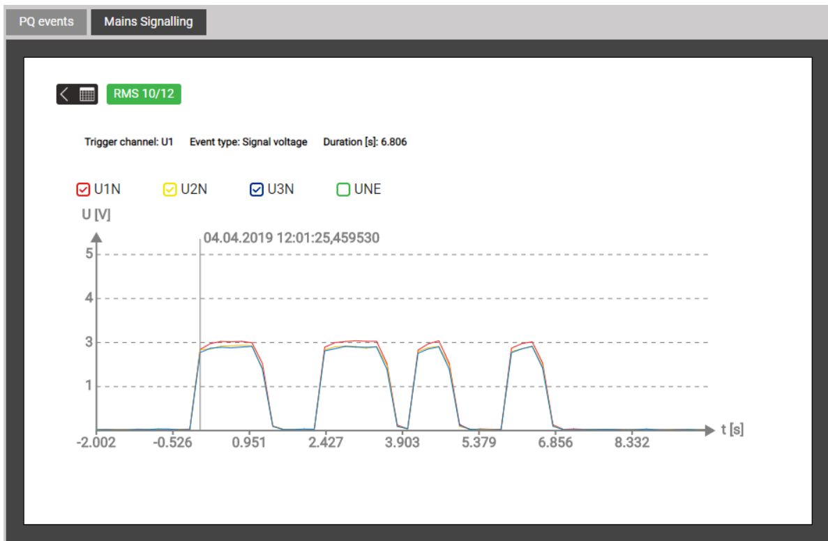
Recognized sequence on the ripple control frequency
