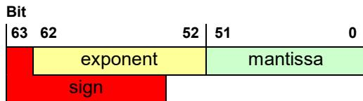
Example: Reading voltage U1N on register address 102 of device 17 (32-bit float)
