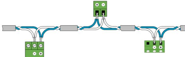
The potential difference of all bus members must not exceed  $\pm 7V$ . Therefore the use of a shield or of a third wire (ref line) for potential equalization is recommended.
