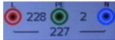
Online voltages are displayed together with test terminal indication. L and N test terminals are used for selected measurement.
