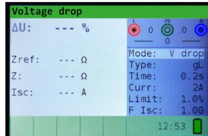
8. Connect the appropriate test leads from the reference point to the instrument to perform phase-neutral or phase-phase line impedance measurement.
