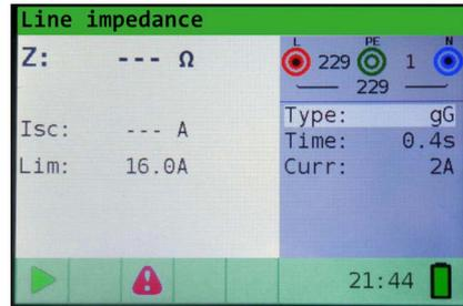
6. Connect the test leads to the instrument, in order to perform phase-neutral or phase- phase line impedance measurement.
