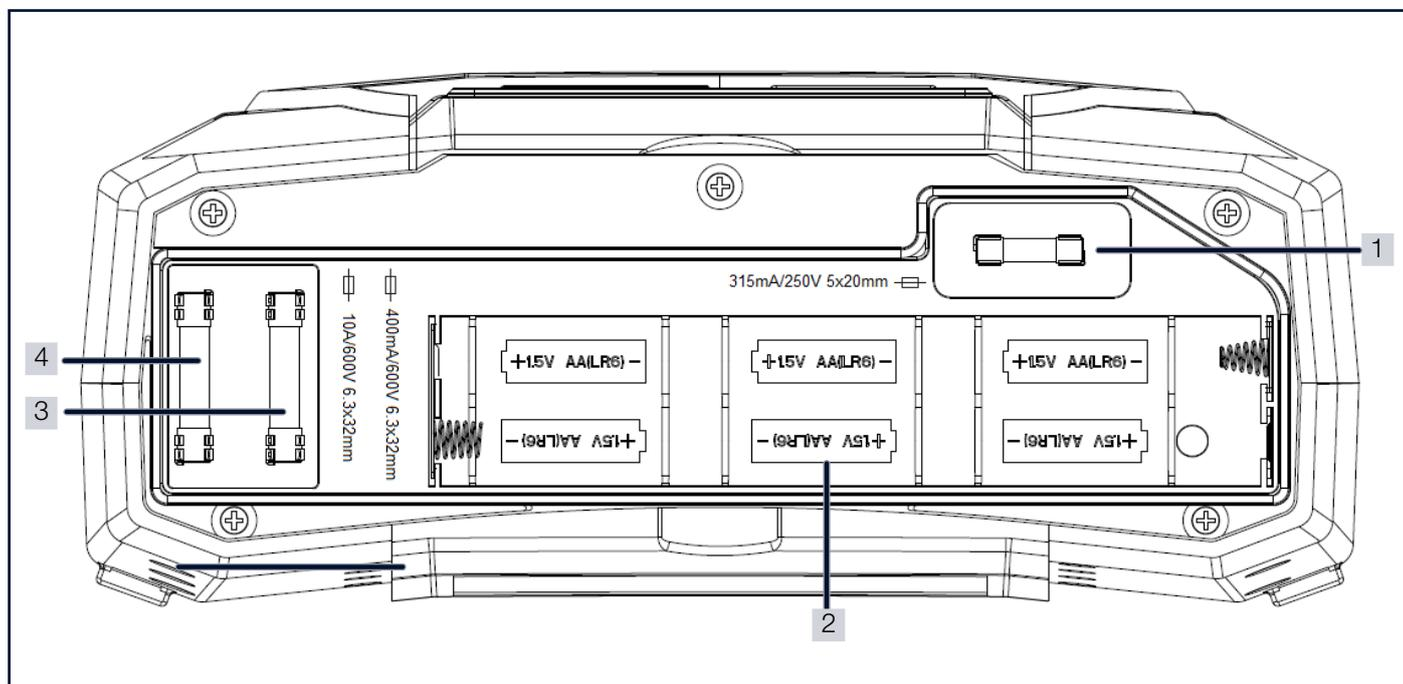
Fig. 4: Battery Compartment
