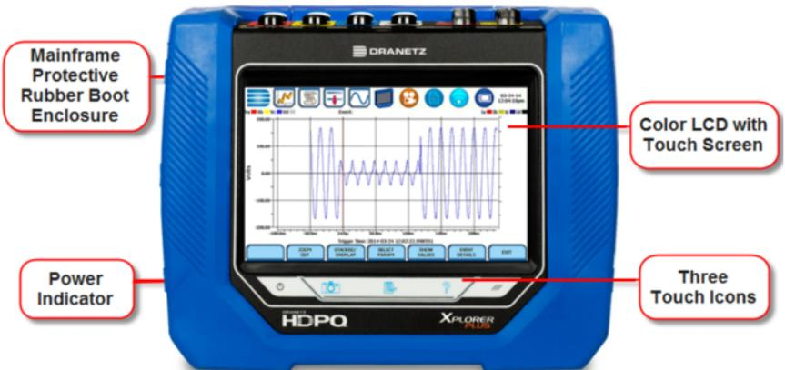
**Color LCD with Touch Screen** – the color LCD has an integral touch screen that is used to select functions for setups, real time meters, and viewing stored data. The color LCD touch screen is operable using the finger and/or a stylus. The touch screen display permits menu selection and alphanumeric data entry. Clean only with a soft cloth.
