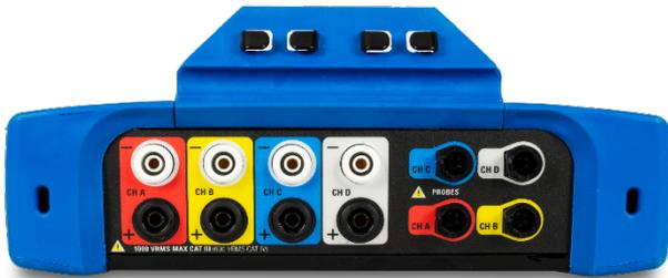
**Voltage and Current Connections** - There are four differential voltage and four differential current channels, which can be wired to measure a variety of circuit configurations. Use only Dranetz voltage leads and current probes for proper operation. Do not exceed the marked maximum ratings.
