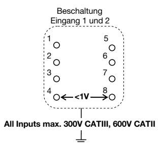
If 2 input sensors or input variables are used, these must be free of potential or galvanically isolated against each other, on principle! Otherwise, the transmitter may be damaged.
