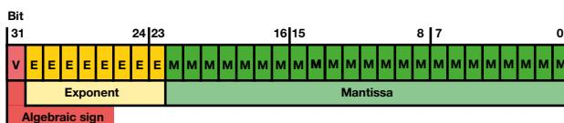
The first register contains Bits 15 – 0 of the 32-bit number (bit 0...15 of the mantissa).
