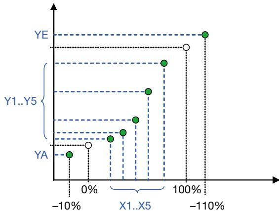
The transmission functions stored in registers OUTSET1 or OUTSET2 constitute information for the PC software to generate the desired transmission function with the table values. This information is irrelevant for the device.
