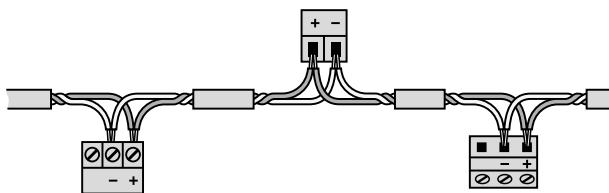
The potential difference of all bus participants may not exceed  $\pm 7V$ . Therefore, the use of a shield or a third conductor (ref line) is recommended to create potential equalisation.
