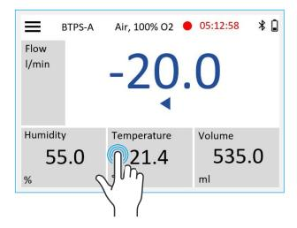
Long press the tile for 1 sec. to open the Edit parameter screen. Here you can select between all available values and units. Use the swipe up / down gesture to scroll through the lists of parameters.
