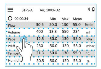
Long press on a row for 1 sec. to open the Edit parameter screen. Use the swipe up / down gesture to scroll through the lists of parameters.
