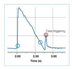
The first two circles indicate the triggers that should be used to measure the volume of this event. However, after the event a small false signal is visible that can be caused for example by switching of valves. In this case a pressure trigger should be used.
