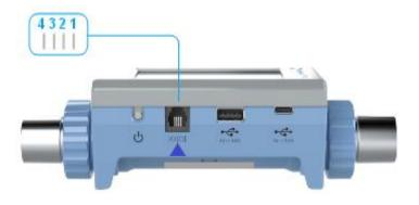
Actuation of the RS-232 port takes place via a special RS-232 cable. If the device shall be actuated via the RS-232 interface, your dealer will be pleased to provide you with a detailed protocol.
