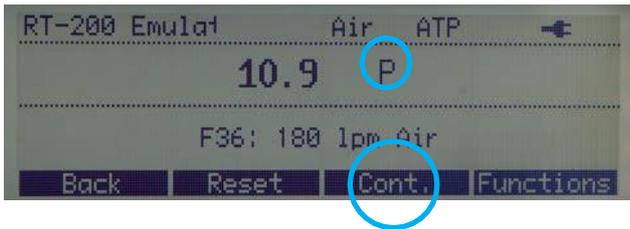
This measuring mode enables you to view the peak values immediately. To switch over to continuous measuring mode select *Cont.*
