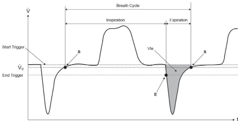
Here too the start trigger should be placed at S and the end trigger should be placed at E.
