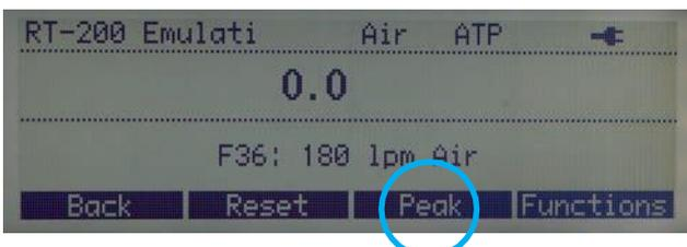
This measuring mode allows you to view on-going measurements. To switch over to the peak measuring mode select *Peak*.
