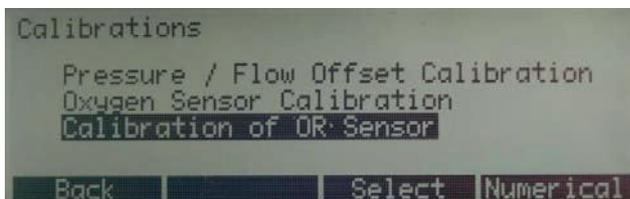
**Note:** If the airway adapter is being replaced, a zero calibration must be performed.
