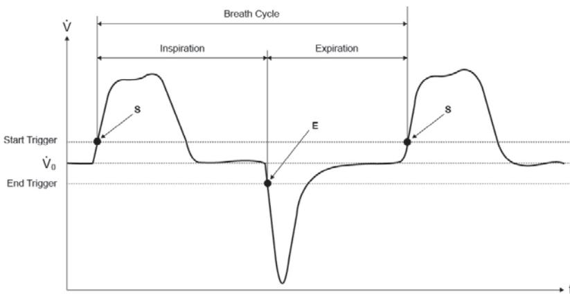
Correct definition of the start and stop triggers is therefore of major importance and it can have a considerable impact on the measurement results.
