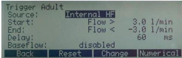
Standard trigger for high-frequency ventilation
