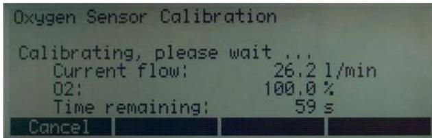
After the start of calibration 100% oxygen and then ambient air have to be applied first, in accordance with the prompt by the device. In both steps it is important for an adequate amount of the corresponding gas to flow through the main measuring channel for a sufficient period of time. For this reason calibration takes approx. 75 seconds per gas. The optimal flow is 20 to 30 L/min and it must not be changed during calibration.
