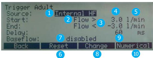
1. **Measurement channel** - Here the measurement channel is selected on the one hand (HF = Flow High channel; LF = Flow Low channel). On the other hand you specify whether internal readings (pressure or flow) will be used as triggers or whether an external trigger is to be used (→5.14.4 Using an external trigger).
