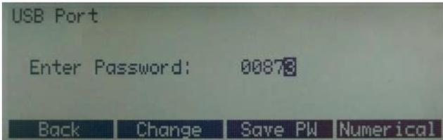
Press **HW activation** to enter. Now various numbers appear which can be selected with the arrow buttons. With **Change** each one can be set to the required value and applied with **Save**.
