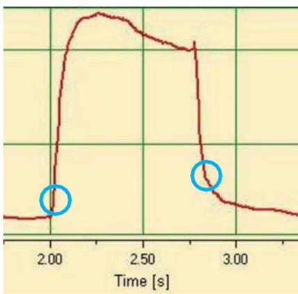
Now here the standard triggers can again be used for the pressure curve: (> 1 mbar/ < 1 mbar).
