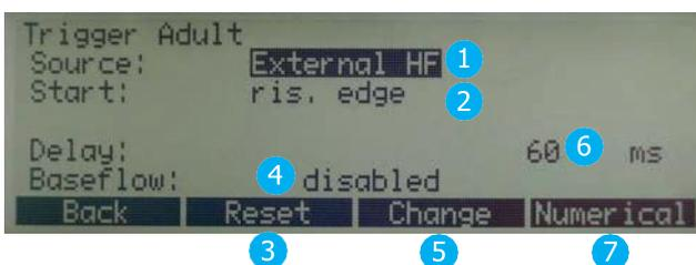
1. **External** - For volume calculation an external trigger signal is used (4.4.3 External trigger).
