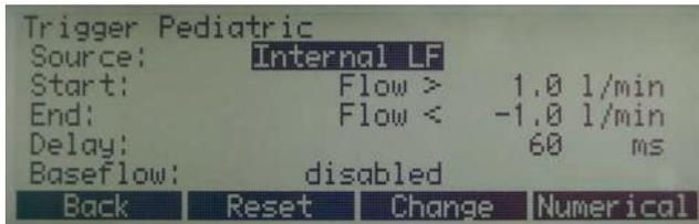
**Note:** The measurement of paediatric ventilation takes place using the Flow Low channel. The required pressure measurement is performed using a tee on the Pd<sub>diff</sub> port.
