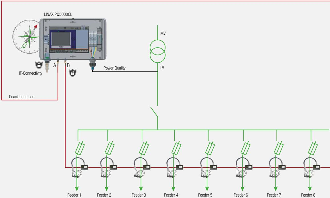
Variant 1: In field housing for wall mounting (built-in power supply for Current Link modules)
