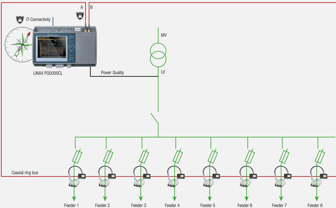
Variant 2: Top-hat rail mounting (additional power supply for Current Link modules required)
