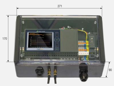
PQ5000CL in field housing with TFT display
