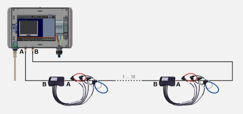
LINAX® PQ5000CL-3 in field housing with connected Current Modules 3PN
