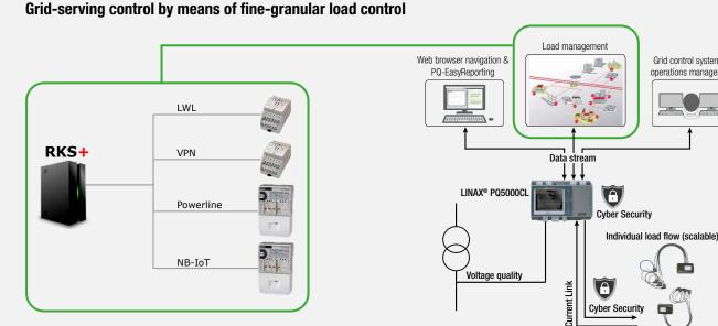
The accuracy and versatility of the Camille Bauer meters extend the RKS load management system into an intelligent, fine-granular network control system. In the event of critical network conditions, the measuring devices
