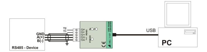
By inserting an external bridge between T1 and T2 terminals, the terminator of the RS485 line is inserted. In case of long connections or noisy environments, it is advisable to use screened cables for the RS485 line.
