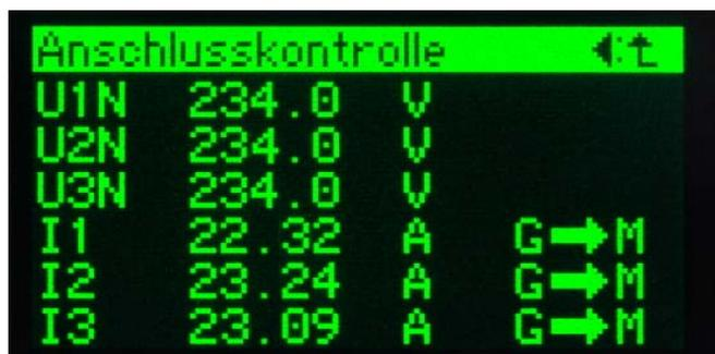
The screenshot shows a terminal window with a green header bar containing the text 'Anschlusskontrolle' and a cursor icon. Below the header, there are six lines of data. The first three lines show phase voltages (U1N, U2N, U3N) all at 234.0 V. The next three lines show phase currents (I1, I2, I3) at 22.32 A, 23.24 A, and 23.09 A respectively. To the right of the current values, there are three arrows pointing from 'G' to 'M', indicating the direction of energy flow.
